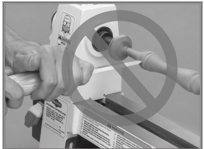
Figure 6. DO NOT cut without using tool rest.
